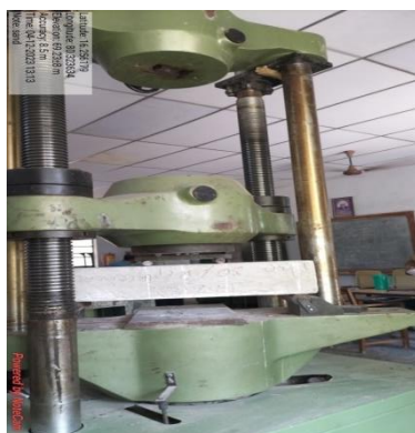
Fig.8 Test setup for Flexural Strength
