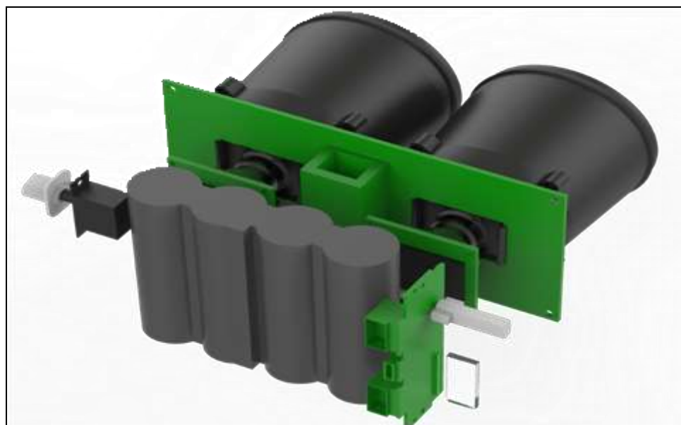
Figure 1: Proposed design of Pupilometer
