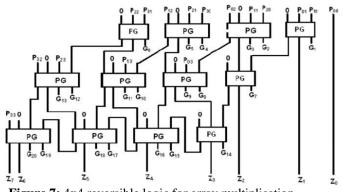
Figure 7: 4x4 reversible logic for array multiplication
