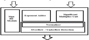
Figure.9: Block diagram of FP Multiplier
