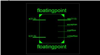
Figure.18: RTL Diagram of reversible logic for FP multiplier
