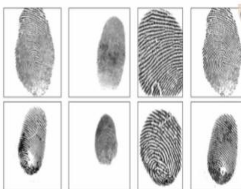
Figure 5: An illustration of a fingerprint scan from LivDet 2015, with authentic samples at the top and fake ones at the bottom. The following Biometrika samples are available: Crossmatch, Digital Persona, Green Bit, and Devices.
