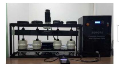
Figure 15: Represent chewing simulator machine (Robota)
