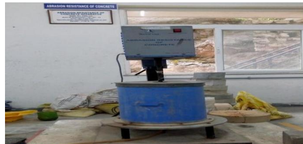
Figure 11 Abrasion testing of concrete
