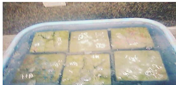
Figure 7 Specimens in HCl solution
