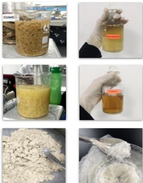
Figure 1. Figure shows the observations on each process of cellulose extraction: (a) OCC during first NaOH treatment; (b) Removal of hemicellulose; (c) OCC during first NaOCl treatment (d) Removal of lignin; (e) OCC after 3 repeated times of NaOH and NaOCl treatment; (f) OCCC formation upon drying
