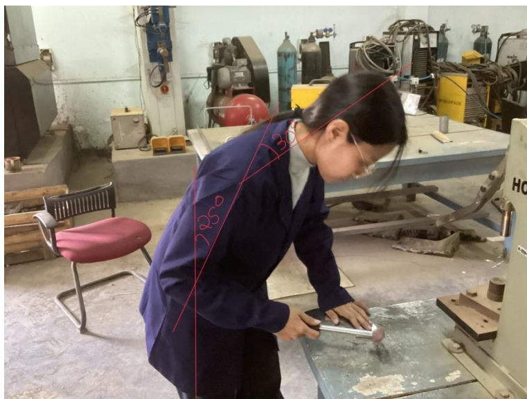
Fig-5: RULA score of 3-4 while preparing a joint using sheet metal work
