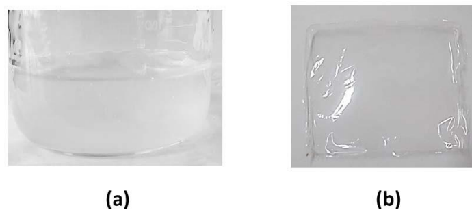
Figure 7: Preparation of Chitosan-based: gel (a), and film/membrane (b) [28,30,31,35]
