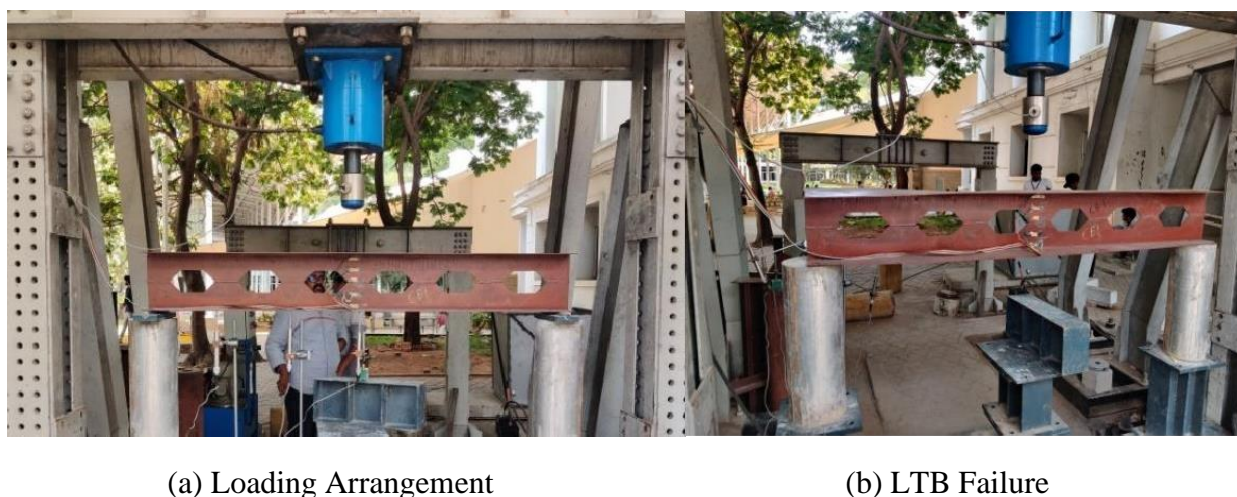
Fig. 9 Loading Arrangement and Failure
