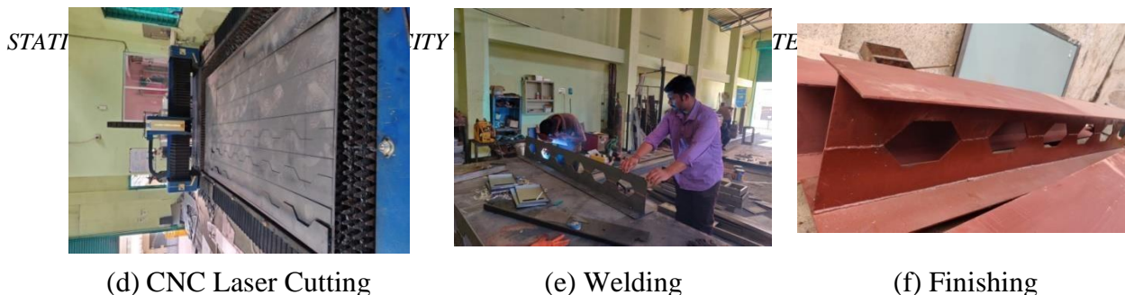
Fig. 8 Preparation of Castellated beam
