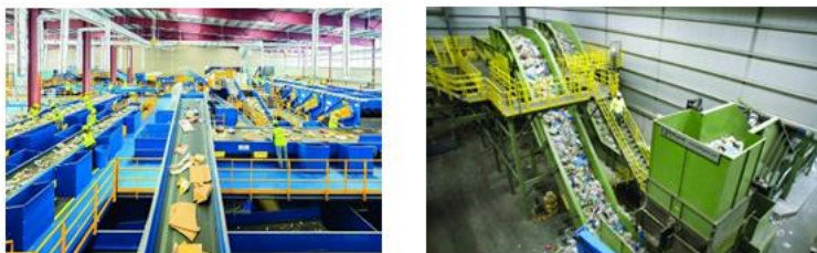
Figure (2) Pictures of the waste sorting station and environmental landfill in Al-Ahsa Municipality
