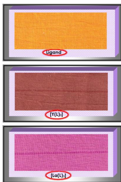
Figure 8. Samples of the textiles' dyeings prepared by using the ligand and its complexes.
