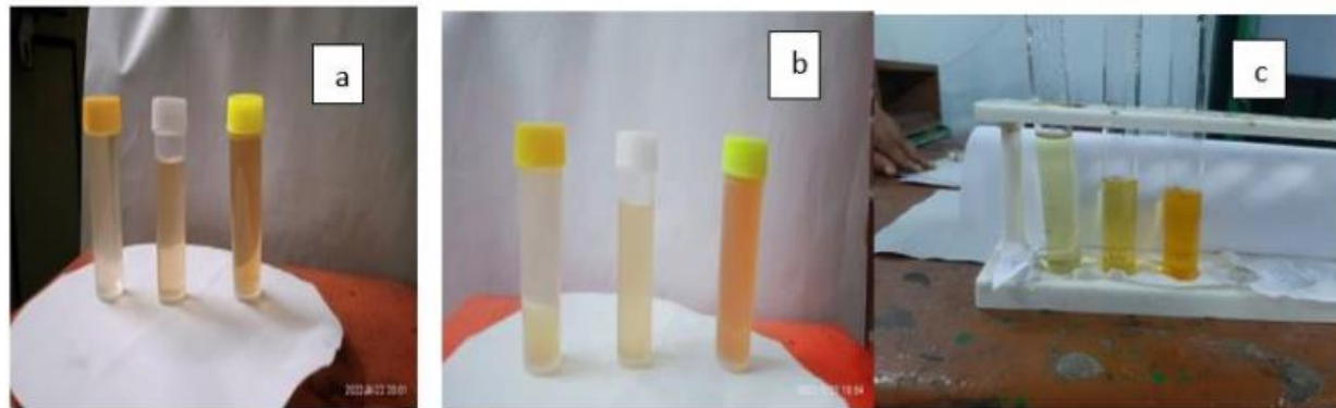
Fig 2: a. Different percentages of MJ Root extract (1%,3%,5%), b. ZnONP 's preparation using different concentrations of ZnSO 4 solutions (1mM,3mM, 5mM) c. ZnONP's preparation using different pH (5,6,10).
