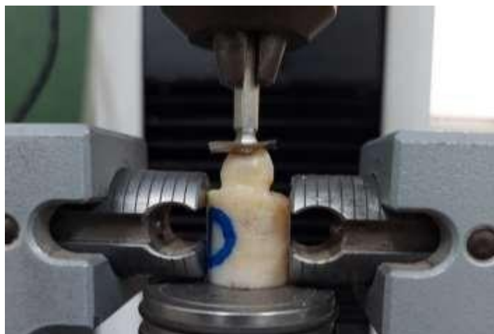
(Fig. 7) Tin foil between the loading tip and the occlusal surface of the restoration
