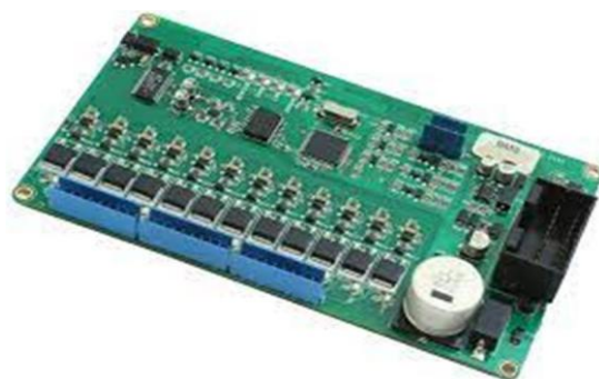
Figure 3: Battery management system
