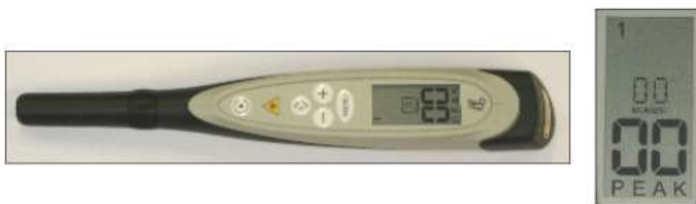
Figure 8. DIAGNOdent pen with the display panel showing the peak and the actual moment measurement
