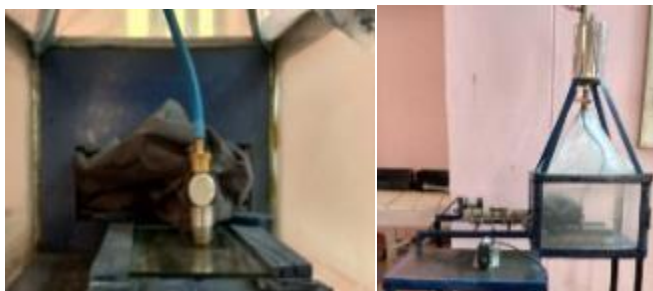
Fig 1: Semi-Automatic Set up of AJM used for the machining
