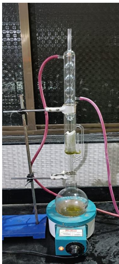
Figure 1: Soxhlet extraction of Clematis triloba using different solvents.
