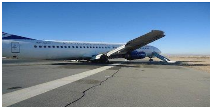
Figure 4. Landing with a technical fault of the landing gear
