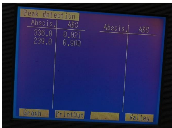
Fig4 : Simvastatin Peak Detection at 239 nm
