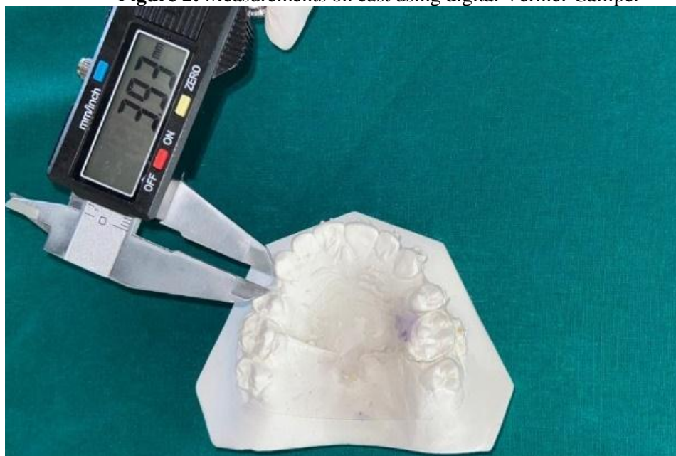
Figure 2: Measurements on cast using digital Vernier Calliper
