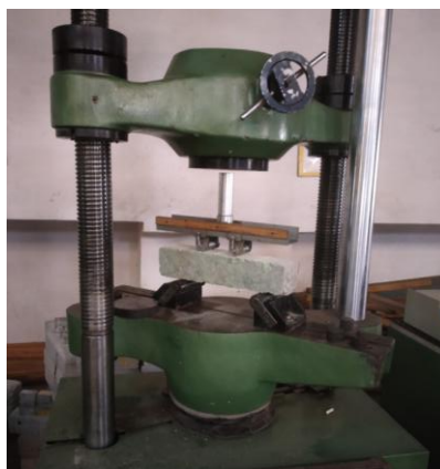
Fig.2 Two point load flexural testing on beam specimen
