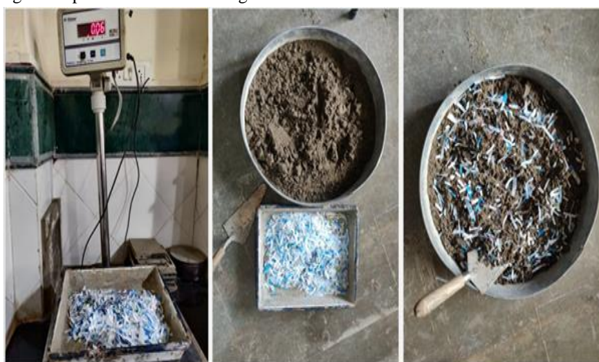
Fig. 2. Marine clay mixed with PW filaments
