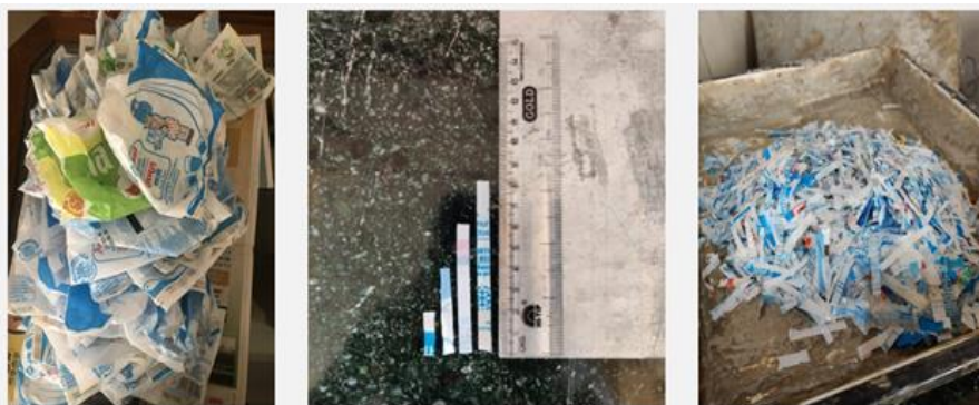
Fig. 1. Soil reinforcing filaments from Milk pouches
