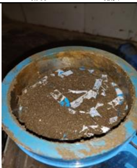
Fig. 3. CBR sample of PW reinforced marine clay
