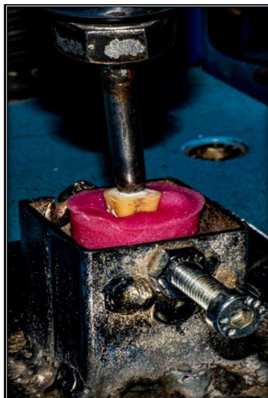
Fig 6: Sample Placed In Universal Testing Machine
