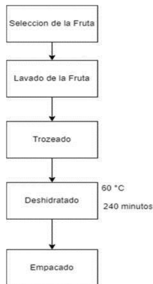
Figure 1: Fruit dehydration process Conducted by: Neppas, Cristian, 2022
