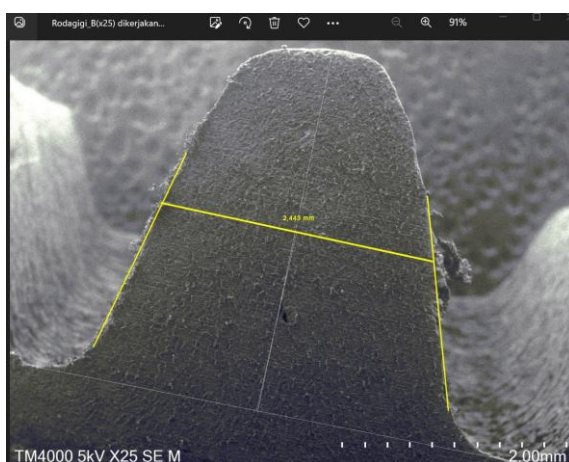
Fig.8 SEM photo for tooth thickness of worm gear ring for Onyx material with oil lubrication (B code)
