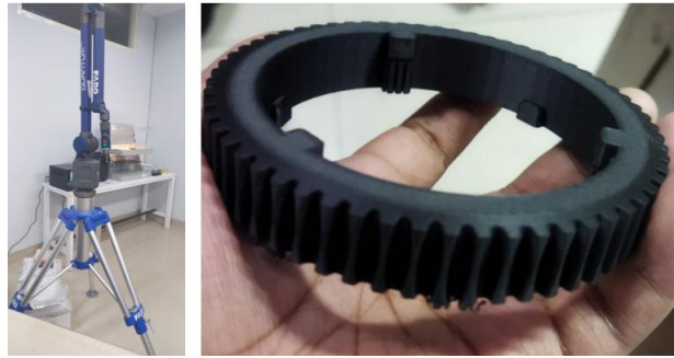
Fig. 3 Three D Scanner (left) and 3D printout of worm gear rings for Onyx composite materials (right) The installation of the worm gear ring on the worm wheel inside the reduction gear is shown in Fig. 4.
