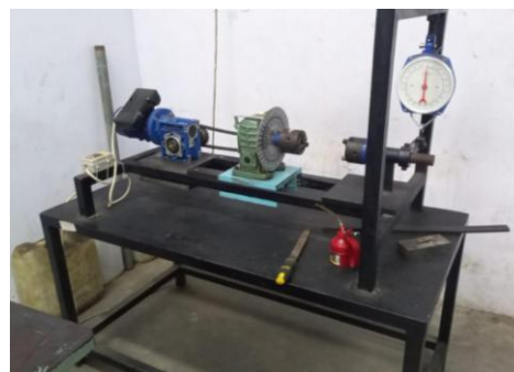
Fig. 5 Torsion Test Machine
