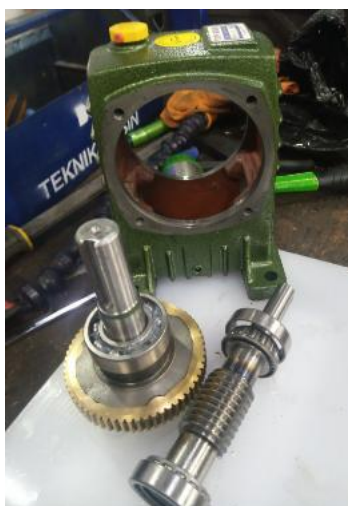
Fig. 2 Worm gear ring made of Brass material
