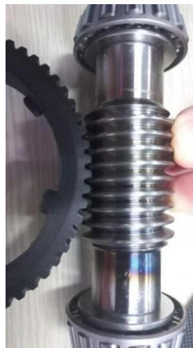
Fig. 4 Installation of the worm gear ring on the worm wheel in the reduction gear
