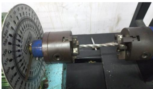
Fig. 6 Torsion test of low carbon steel specimens
