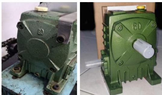
Fig. 1 Reduction gear: (left) Installed on torsion testing machine, and (right) New [17]
