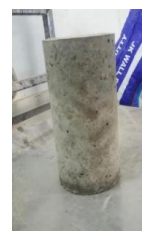
Figure 5: Casted Specimen for the Tensile Strength Test
