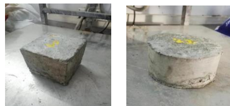
Figure 4: Casted Specimen for the Compressive Strength Test
