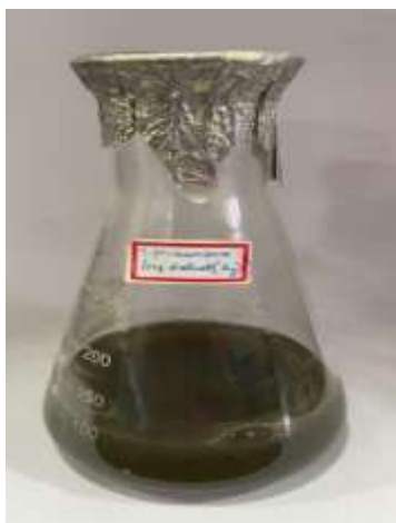
Figure 2: Reduction of silver ions to silver nanoparticles visually identified by color change
