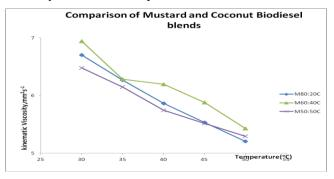
Figure 1. Viscosity of blends of mustard and coconut oil biodiesel
