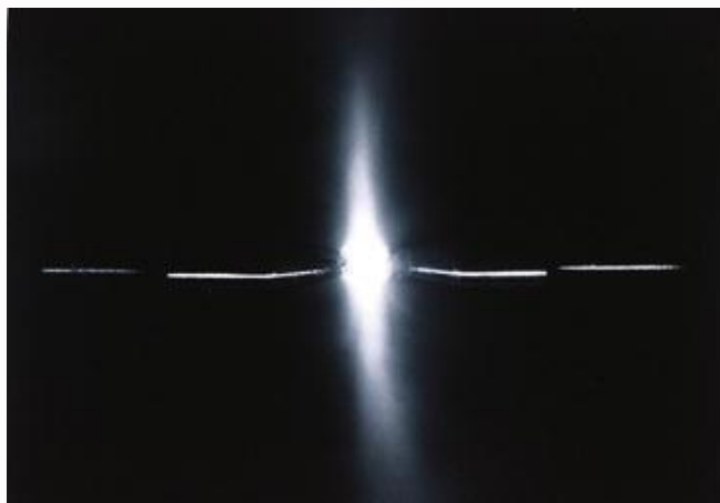
Figure (5): Photograph of a high-voltage discharge between two electrodes immersed in water. (10).
