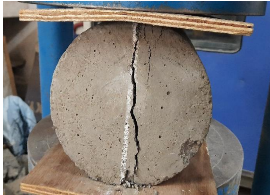
Fig.2: Split Tensile Test on Concrete Cylinder
