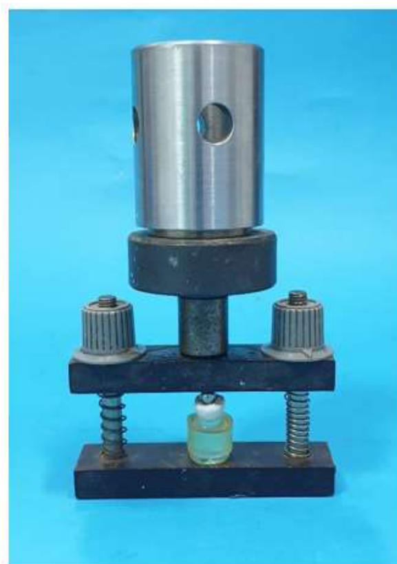
Figure [4] Cementation device holding specimen and applying vertical load
