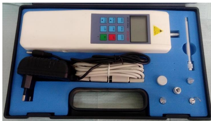
Fig (3) Digital force meter device for retention measurement
