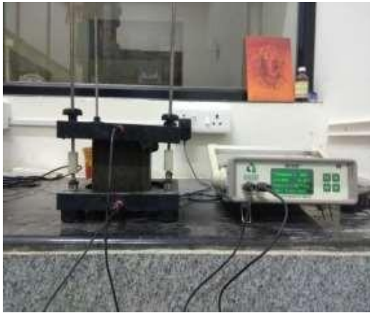
Figure.2 Setup for measuring electrical resistivity of hardened concrete
