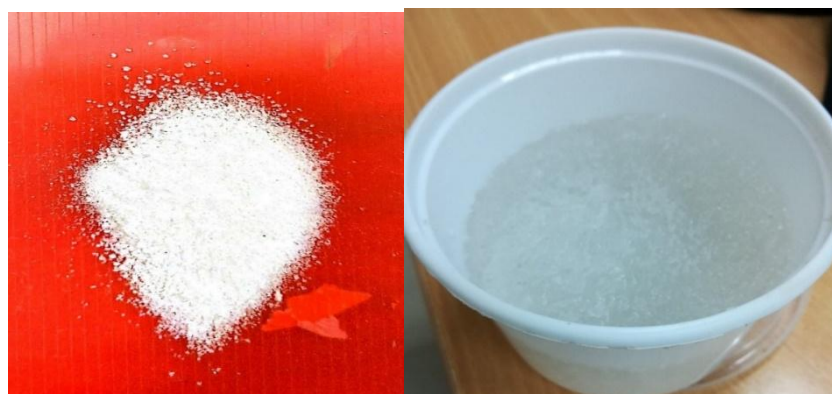
Figure 1: Super absorbent polymer before and after swelling with the addition of water.
