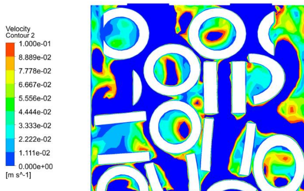
Figure 11. Gas velocity magnitude on the center cross section of the packed column at liquid velocity of 0.4 m/s
