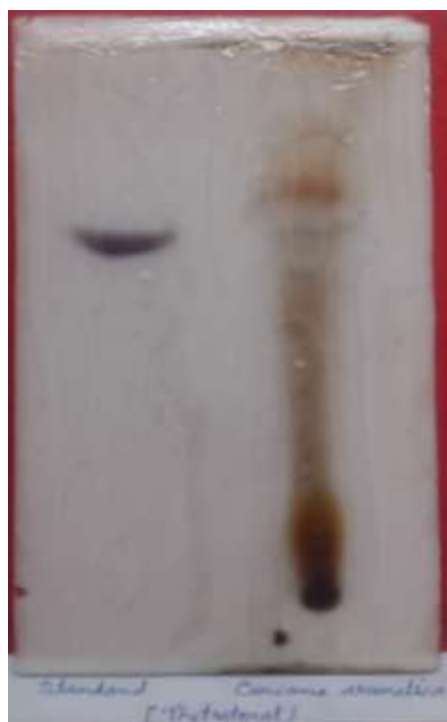
Figure 1: TLC of Phytosterol compounds isolated from Curcuma aromatica rhizome (ii) Alkaloid compounds
