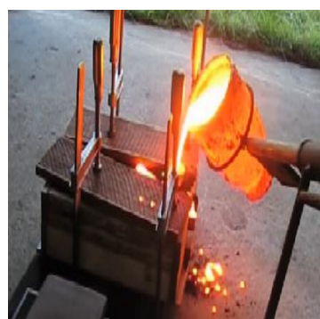
Figure 5. Molten metal pouring in mould
