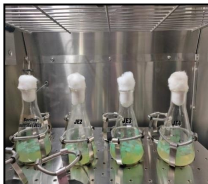
Fig 6: Biodegradation of LDPE film
