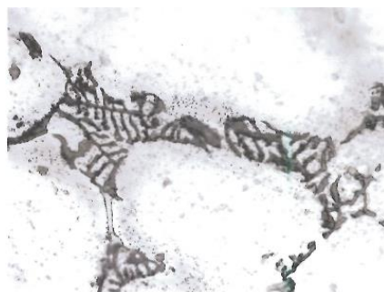
Figure 20. Magnified microstructure at 1000X, Hydrofluoric acid, 15 sec. Source: Own elaboration.
