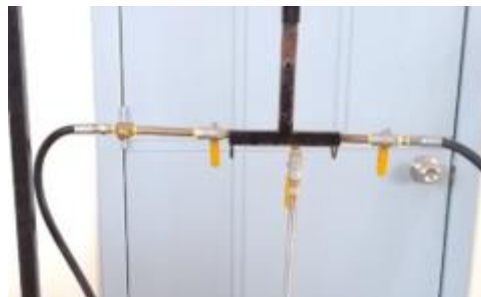
Figure 15: Attachment of the valve system to the mold.
