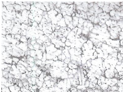
Figure 17. Microstructure magnified at 100X, Hydrofluoric acid, 15 sec. Source: Own elaboration.
