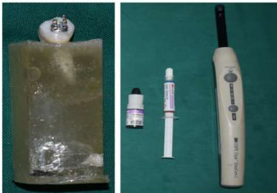
Fig.1: (a).Extracted teeth mounted on acrylic block (b). Transbond MIP and light cure composite (3M Unitek, Monrovia, CA, USA)
