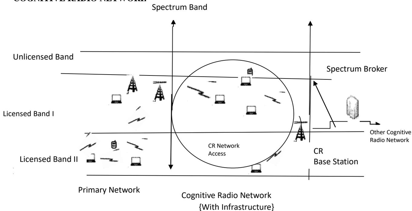
Fig.1: Infrastructure-Based CR Network Architecture
