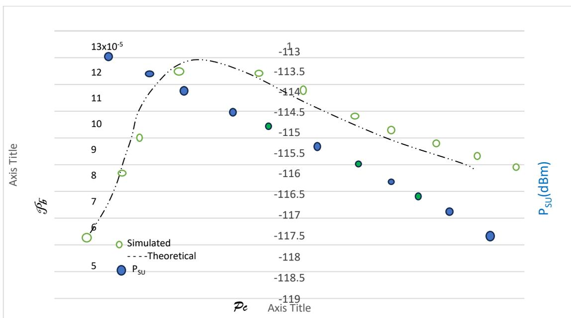
Figure 06. PU performance with a fixed SU value PY = .9 and a range of SU (Pc, PSU ) operating pairs on the 2nd-order polynomial boundary.
