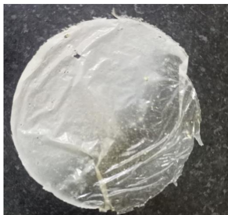
Fig. 5.4) PHA Biopolymer film produced using thin stillage (TS)
