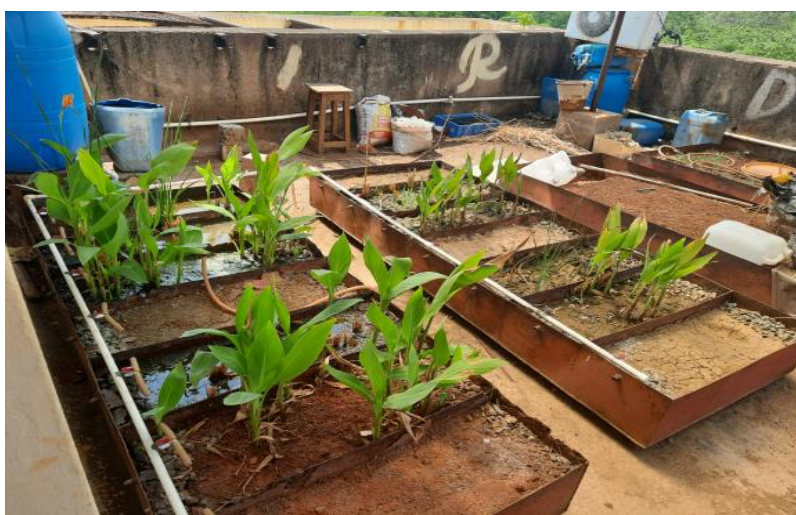
Figure 1: View of Horizontal subsurface flow Constructed wetland (pilot scale), A. Cross section B. Site View
