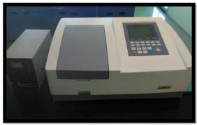
Figure 2: Schematic diagram of UV-Visible Spectrophotometer working and an UV spectrophotometer
