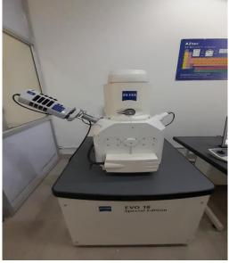
Figure 3: Schematic diagram of SEM working and its photograph
