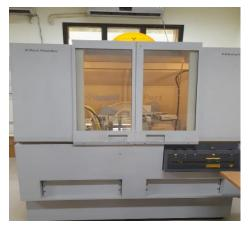
Figure 4: Schematic Diagram of X-ray Diffractometer and its photograph
