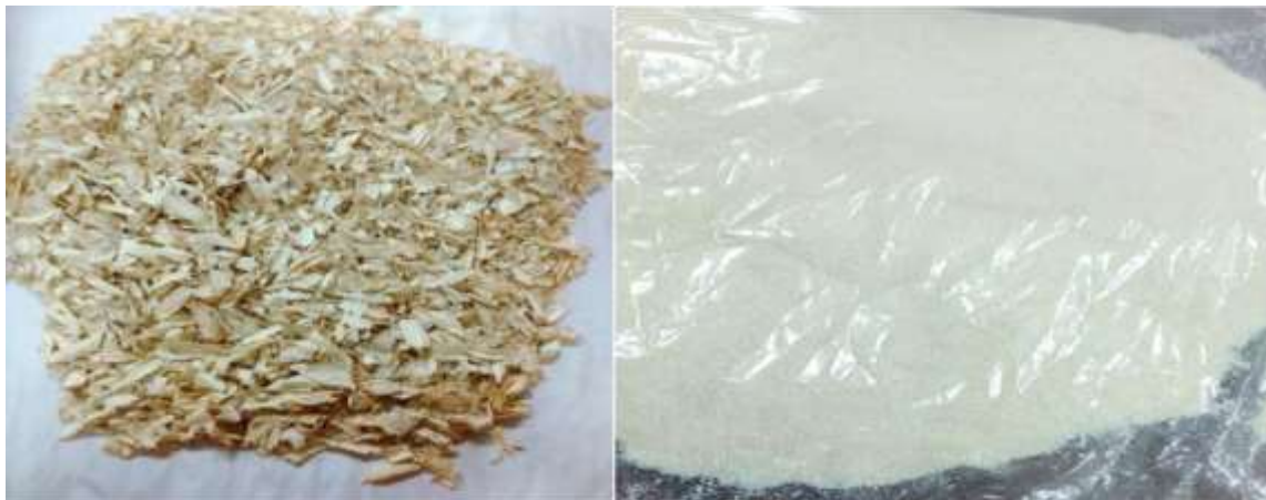
Figure 1: Chemically treated shells and powdered chitosan from shells
