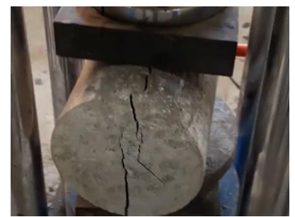
Fig: 4 (a) Filling of concrete mould, (b) After curing of cube and (c) compressive test
