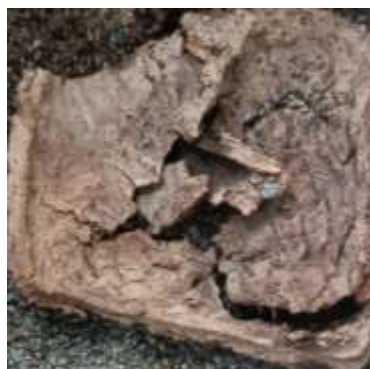
Fig 7. Dried Sludge with cracks
