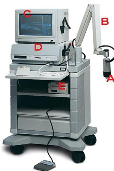
Fig. (1): The current UBM—P45 workstation (Paradigm Medical Industries, UT, USA). A: Ultrasound transducer and probe; B: Articulated arm; C: Computer monitor; D: Main processing unit; E: Printer (21).
