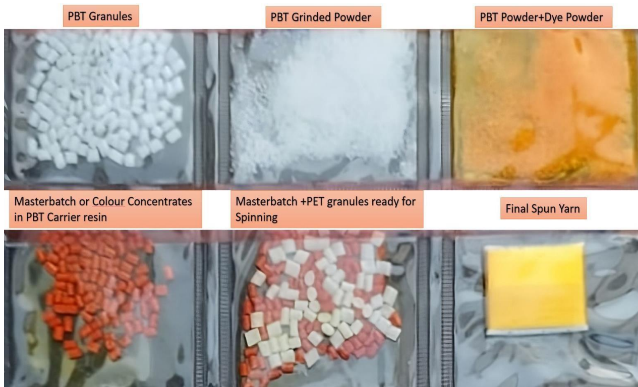
Figure 4: Process Steps – Polyester spin Dyeing (Mass coloration)
