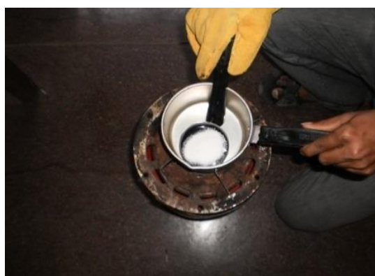
Step 2: Addition of Polymer Modifier
